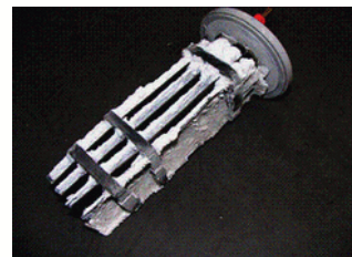
Scaled Chlorinator Cell High TA leading to high pH
